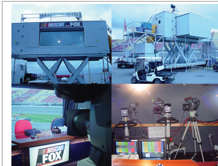
Figure 3.40 People outside the industry sometimes ask if the production truck also has a studio. There are studio trucks. If announcers and commentators need to be close to the pits for a car race, this movable announce booth can be used. The booth is on scissor lifts that raise it approximately 15 feet into the air. The expandable section is where the cameras are placed. Two of the cameras are robotically controlled, while the third can either be manned, or locked down on a wide shot. Since race venues are usually very large geographically, and this truck is often far from the main television compound, it also acts as a video and audio termination point. That means microphones and miscellaneous video sources can be run to this truck, which multiplexes the various signals onto a few fiber runs back to the main truck compound.
