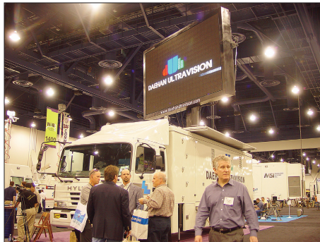
Figure 3.42 This 9.5-ton truck's output is not to satellite or fiber, but to the 149 square foot display on a pneumatic pedestal above it. The display has close to 300,000 LEDs, and folds in half (top rear against bottom rear) when it is stored parallel with the sides of the truck. The truck has only VTR playback capability, or can take an external feed.
