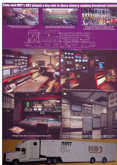
Figure 3.30 Sony/NMT brochure highlighting one of NMT's HD trucks. HD trucks are the toughest to build, maintain and operate of all remote trucks on the road. The equipment takes up more space, consumes more power and generates more heat. The productions can also be more involved, as clients often want HD and SD out of the truck at the same time.
