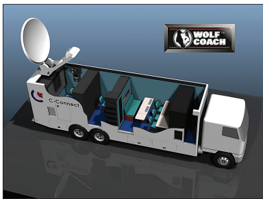
Figure 3.35 A cutaway view of a production/Ku uplink truck. The front compartment is production, the middle is audio, and the rear is for video and the satellite uplink equipment. (Source: Wolf Coach)
