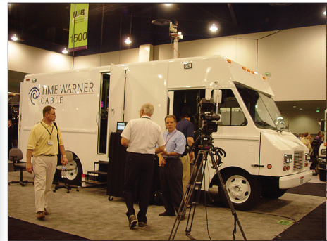
Figure 3.34 Step van that can accommodate up to five operators, but is laid out so that only a couple inside the truck are necessary. This truck also has its own 7kW/110V/60A generator.
