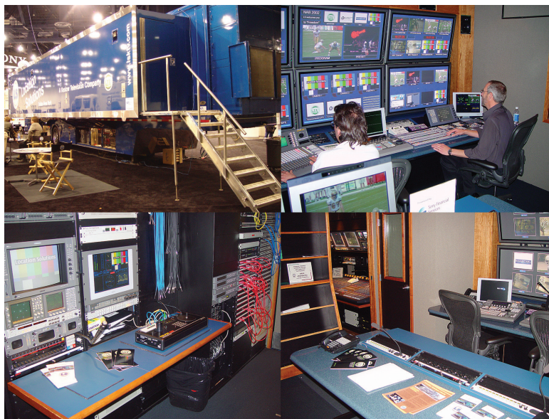
Figure 3.39 A new breed of remote truck, this truck was not designed to do "classical" remotes, but rather to support other trucks at a venue. The compartment in the upper right can be used as a high-end production suite, as master control, or as a release center when a group of trucks are needed for a production. The bottom right photo shows more editing stations (right side), an extensive audio compartment (left), and even an announce booth (door at center). The bottom left photo is transmission, and a quality assurance (QA) station. This trailer has extensive computer networking throughout, and over 5000 feet of fiber optic cable installed.
