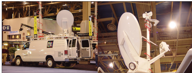
Figure 3.37 The ENG/SNG truck shown above and to the left can use microwave or satellite paths back to the television station. Because the truck is physically smaller, the satellite dish it carries will be slightly smaller than ones found on larger trucks, which results in slightly less gain for the satellite signal.
