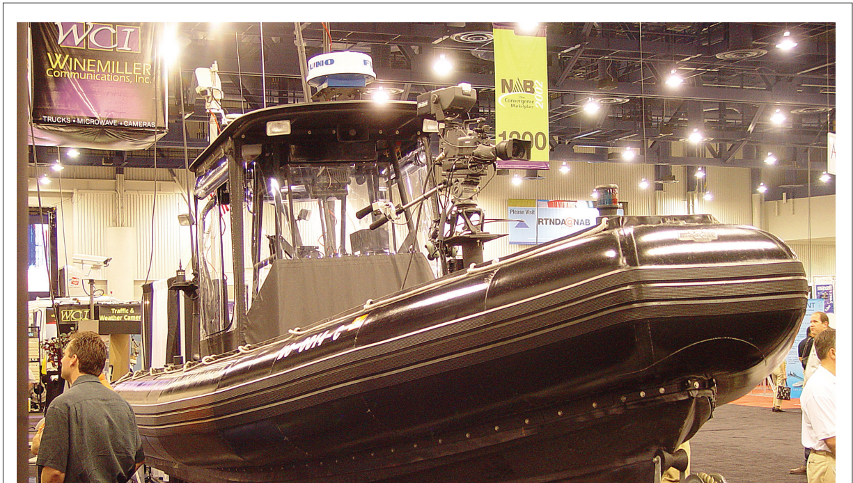
Figure 3.44 Finally, a remote boat! This 4900-pound, 24-foot Zodiac rigid inflatable boat, manufactured for the U.S. Navy, is intended for use on water-based reality shows. The camera is mounted on an M-60 gun mount.
